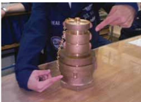
Overboard Discharge Assembly
